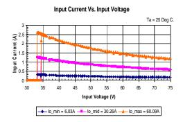
iHA48060A012V-001 Typical Input Current vs. Input Voltage Characteristics at Ta=25 degrees.
